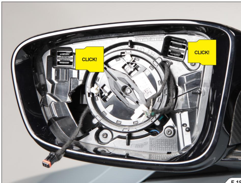
3. Reinstall mirror glass into of both side view mirrors; check vehicle manufacturer work shop manual for details (F 20, 21, 22).
