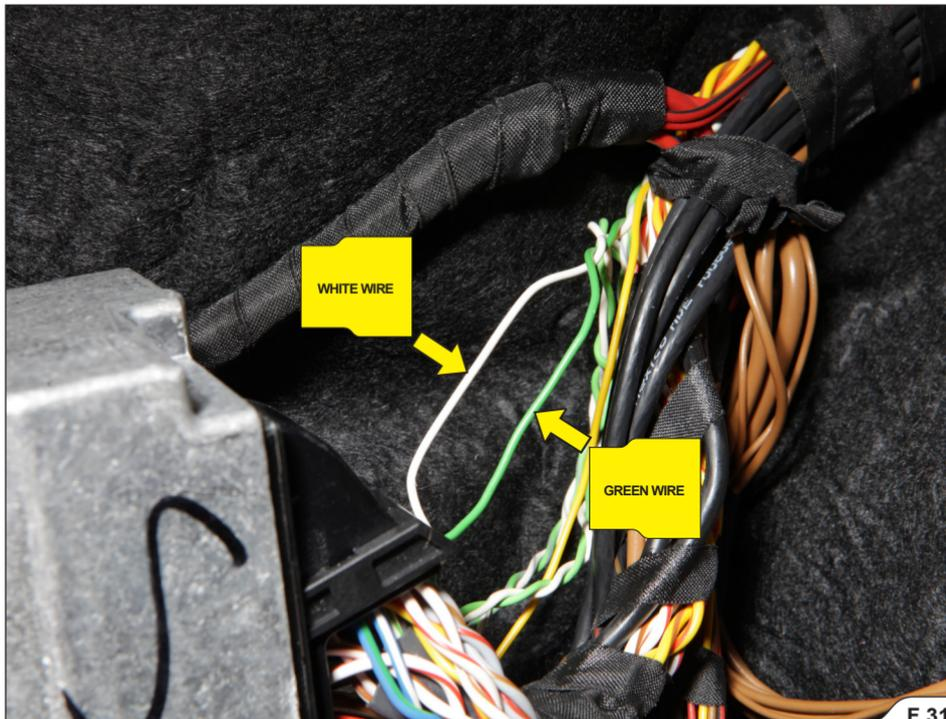
**!** IMPORTANT: test the Control Kit; in case it doesn't function correctly, use another pair of WHITE-GREEN wires for CAN sniffer (F 31, 32, 33).
