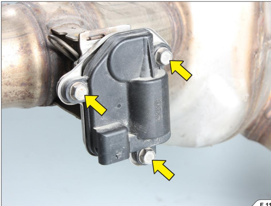
5. Unscrew the marked bolts and nuts and remove all parts of the muffler heat shield (F 12).
