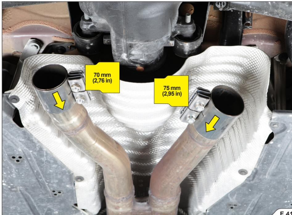
8. Obtain **two original BMW** exhaust valve actuators (**part nr. 18 30 8 686 640**) from your local BMW dealership. Assemble the stock rubber brackets and two original actuators onto the Akrapovič muffler, using heat shields and bolts from Akrapovič installation kit (**F 42, 43, 44, 45, 46, 47**).
