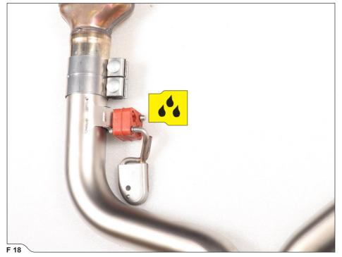
For SHORT Link Pipe only: carefully install the Link Pipe onto the vehicle; tighten the rubber brackets onto the chassis, tighten the stock flanges (using stock nuts), align the pipes in respect to the chassis, align the clamps as shown and tighten them to the specified torques (F 19, 20, 21).
