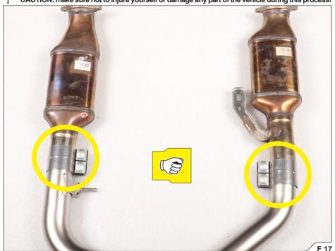
INSTALLATION TIP: for easier mounting, lubricate the original rubber bracket (WD40 $^{(8)}$ )\*. \*WD-40 $^{(8)}$  is a trademark of the WD-40 Company.
