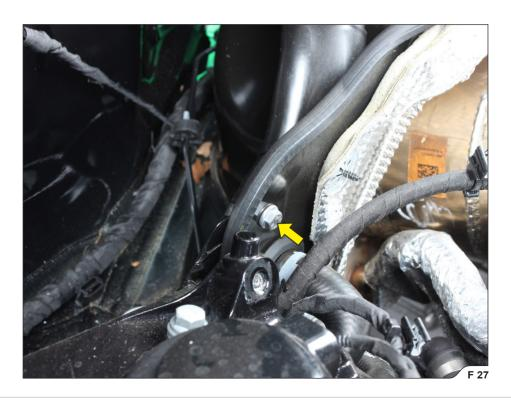
For vehicles with OPF/GPF only: undo the market clamps, remove the tubes off the sensor, disconnect the sensors' electrical connectors, unscrew the marked bolts and remove sensors, on both sides of the engine compartment (F 28).
