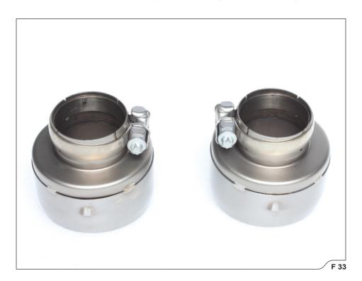
12. Install the tail-pipes onto the muffler outlets. Adjust, rotate and center them in respect to diffuser's cut oats and according to your personal preference; tighten the tail pipes' clamps to the specified torque (F 34, 35, 36).
