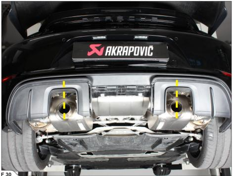
8. **For clamp type fitting muffler vehicles only:** loosen the market muffler's bracket bolts, adjust and center the muffler so that muffler's outlets are in the centers of diffuser cut outs, then retighten the bracket bolts (F 27, 28, 29).
