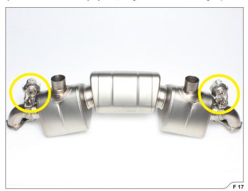
MPORTANT: before tightening the actuator's nuts, adjust and align the actuator's heat shields in such a way, that the connection of vacuum tubes is possible!
