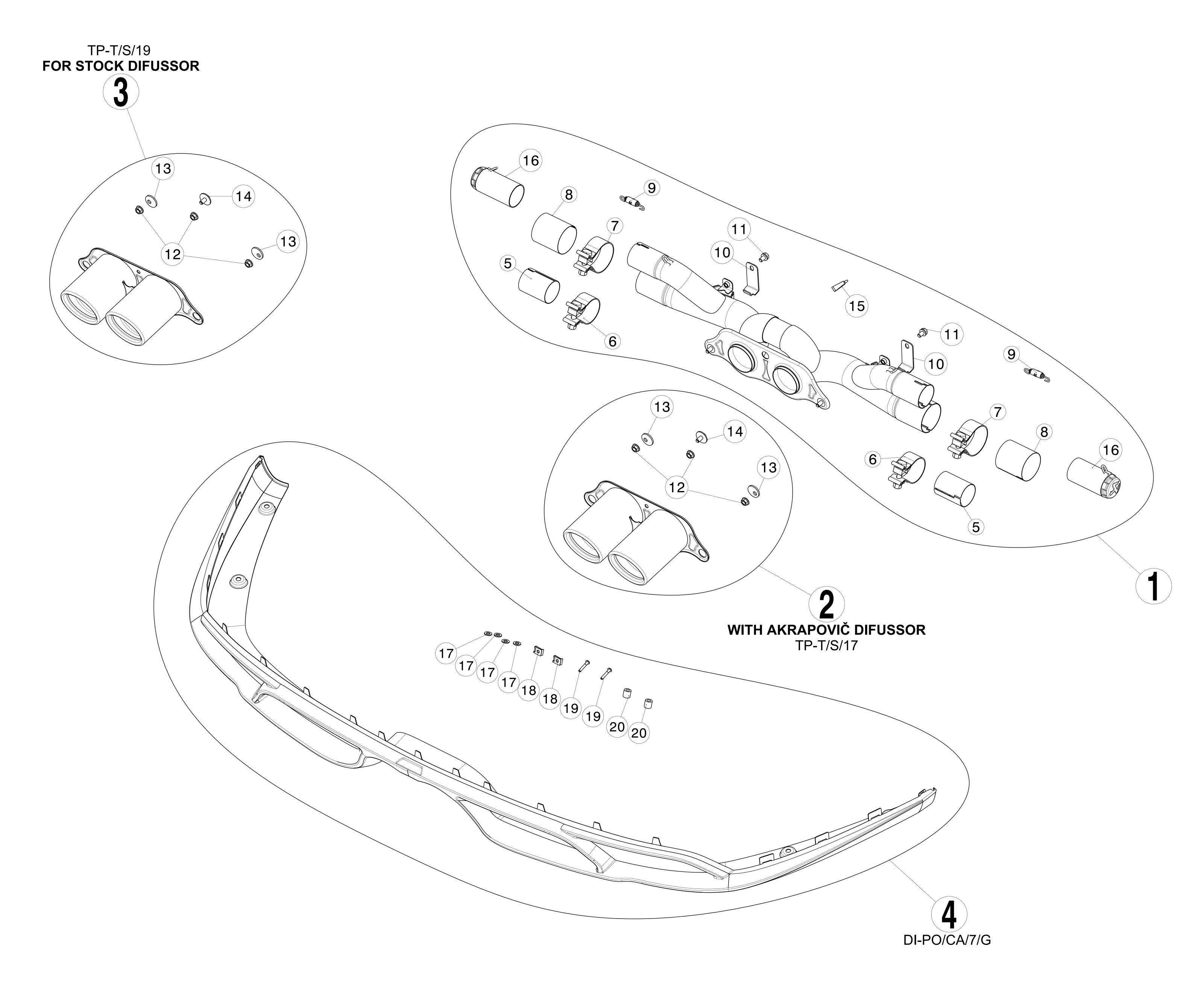
Note: Diffuser DI-PO/CA/7/G has to be used with tail pipe set TP-T/S/17
